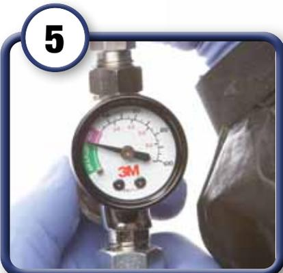
5 Set air pressure at 20 psi for 2<sup>nd</sup> stage (air and fluid flowing)
