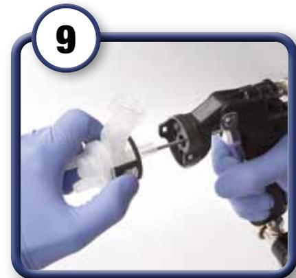
Remove atomizing head - be sure to pull trigger back and pull the atomizing head straight out from the gun body to avoid bending the fluid needle.
