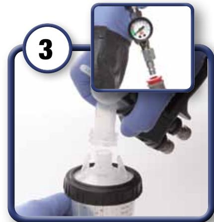
Attach 3M™ PPS™ cup filled with primer and attach compressed air hose.
