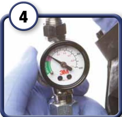
4 Set air pressure at 30 psi for 1<sup>st</sup> stage (only air flowing)
