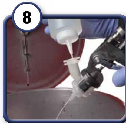
Flush out atomizing head with appropriate solvent until the atomizing head is clear of primer.
